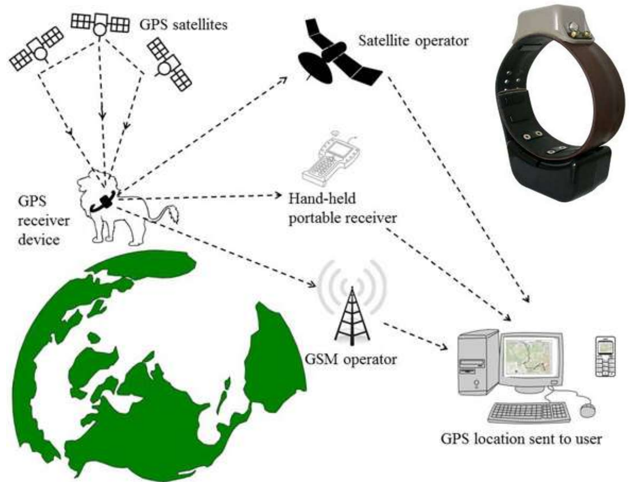
Figure 1. Remote data transfers for GPS-based tracking systems use a GSM link, a satellite-based link, or a handheld terminal.
